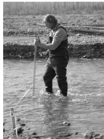
Figure 5. A hydrologist makes discharge measurements on the East Fork River.
