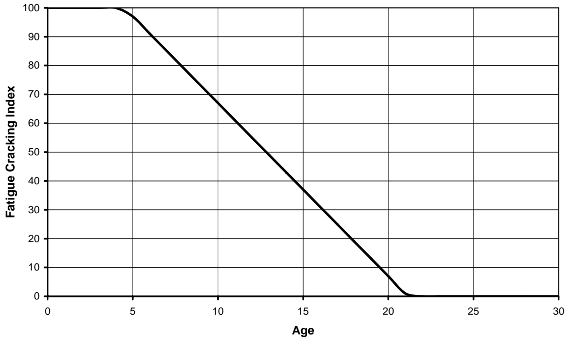
Figure 81. Chart. Fatigue cracking index trend for environmental case wet no-freeze.
