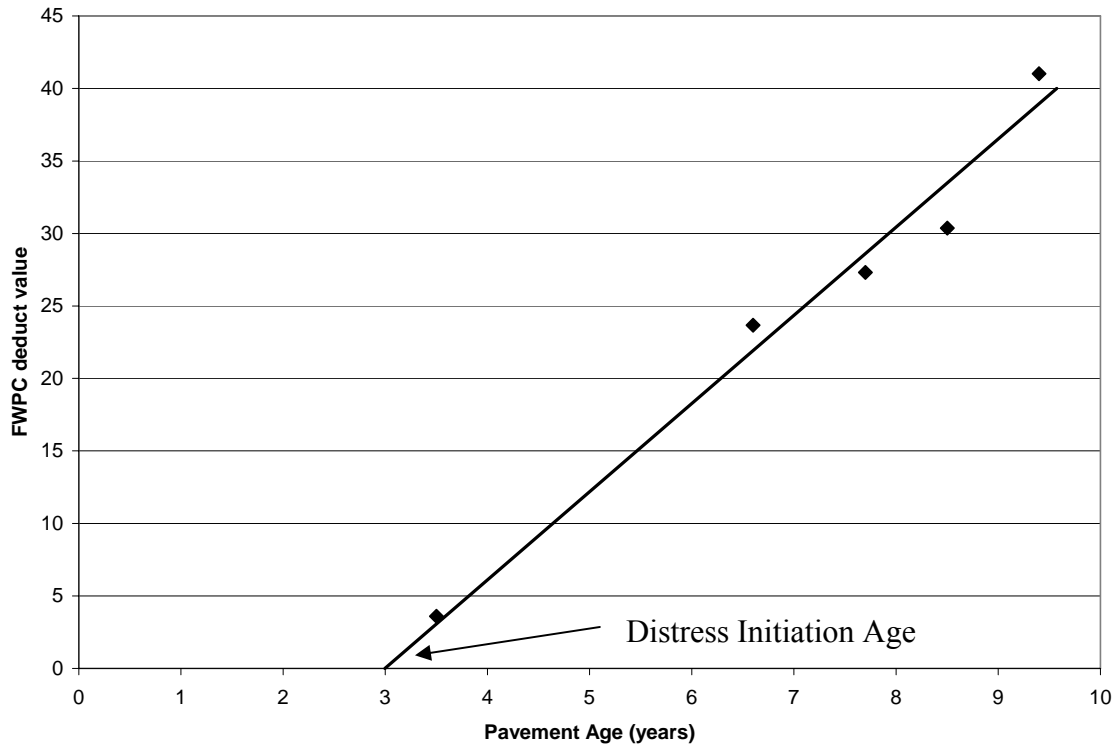
Figure 26. Graph plot. Observed FWPC deduct values for test section 050121 (with regression line).
