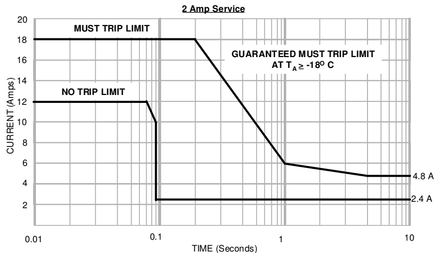
Figure 3-2 SSPC In-rush and Trip Current Limits Curve for 2 A service
