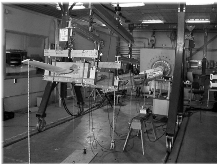
Figure 4.5 Photograph of the ERS-100 Blade Under Load
