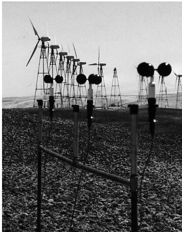
Figure 5. 4 Photograph of the Anemometer Calibration Frame.
