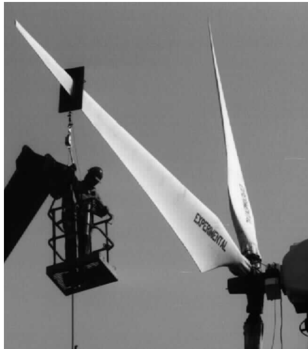
Figure 5. 9 Photograph of Blade Strain Gage Calibration
