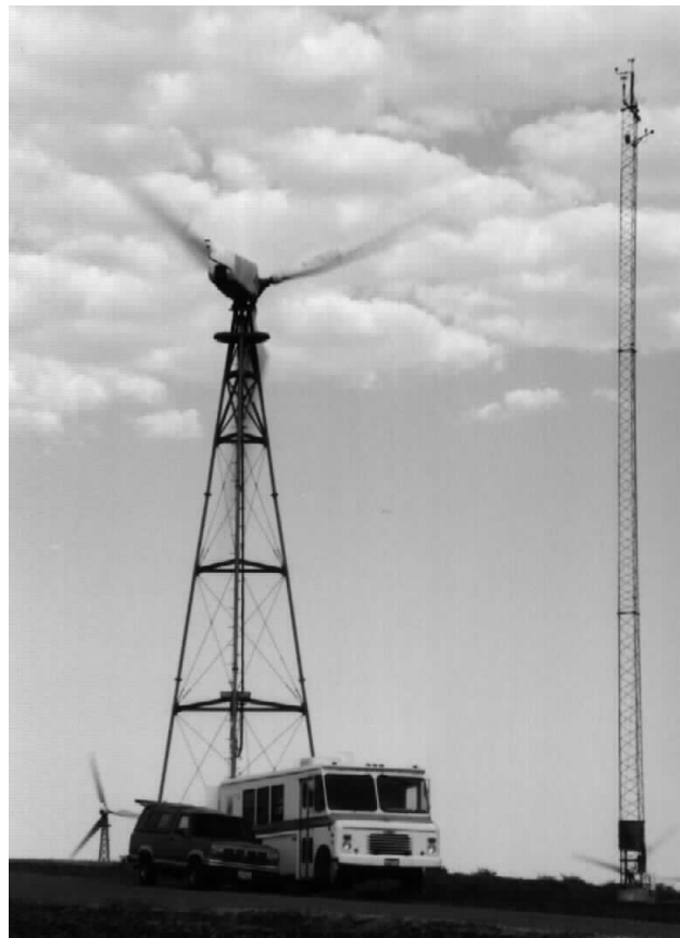
Figure 5. 2 Photograph of the Test Van and Meteorological Tower
