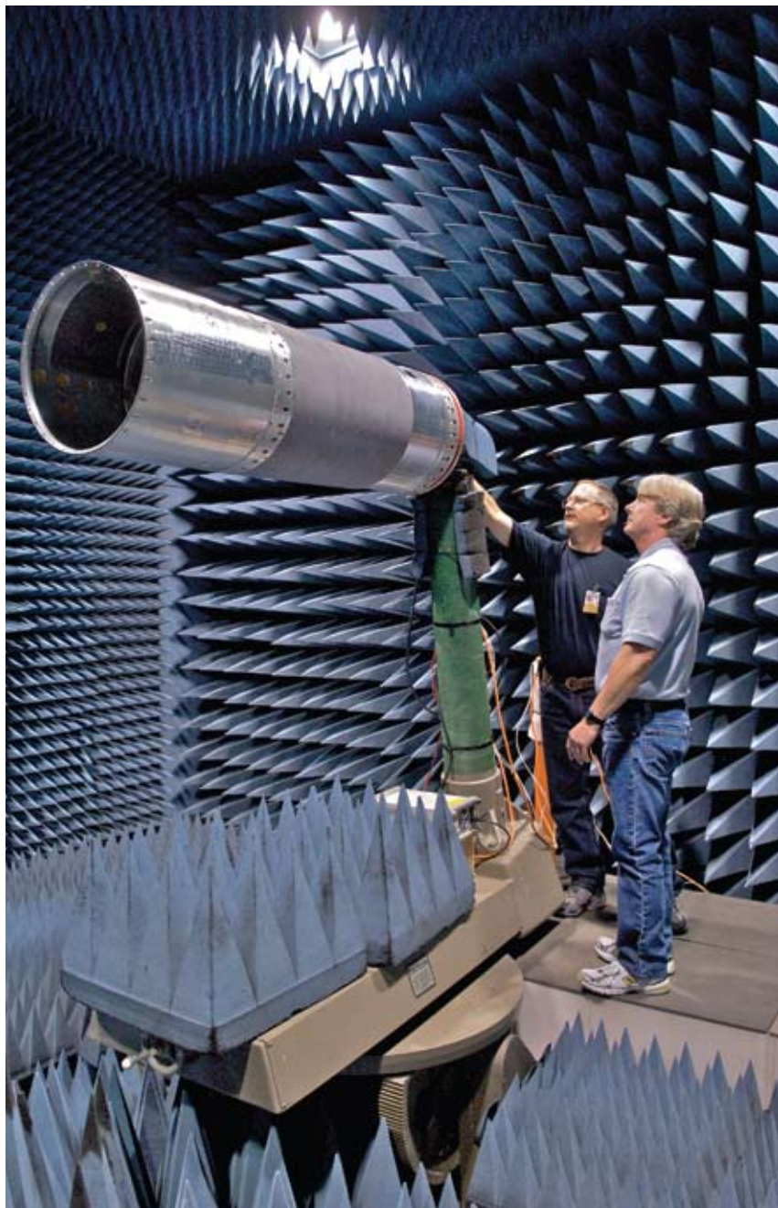
Bruce Smith (right) and Con Duer (left) work on a team to develop a beam-steering phased array at Wallops Flight Facility.
