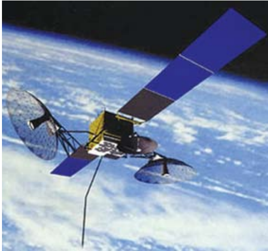
The AFSS effort began with NASA's Low-Cost TDRSS Transceiver, a communication signal relay system that provides tracking and data acquisition services between low earth orbiting spacecraft and NASA/customer control and/or data processing facilities. Bull is principal investigator of a NASA- and DARPA-funded effort that will enable testing of the merger of AFSS and TDRSS systems.
