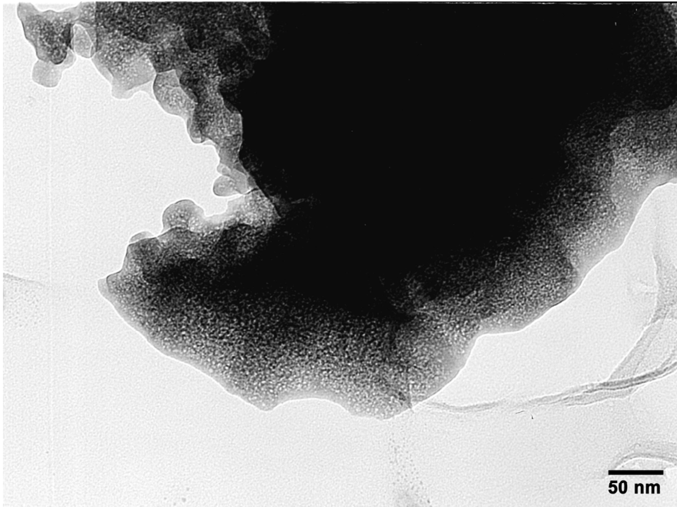
Small, helium bubbles in a single phase, LaNi 4.7 Al 0.3 region
