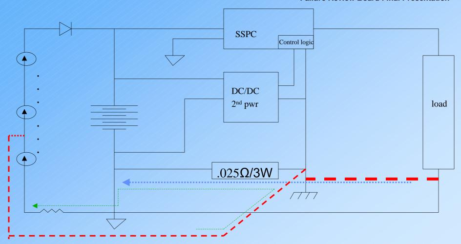
The maximum value of chassis current telemetry is 1A. That accounts for 0.025V of reference shift at the bus return which is not enough to affect a MOSFET gate bias on the SSPC. The chassis current telemetry is negative which means it is flowing from the structure to the bus return. This supports a load return line shorted to chassis.
