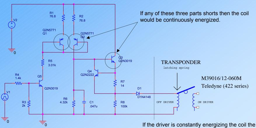
If the driver is constantly energizing the coil the magnetic force will keep the relay latched in the open position. Even if the ON driver overcomes the OFF coil field for the pulse duration, the OFF field will latch it back on.
