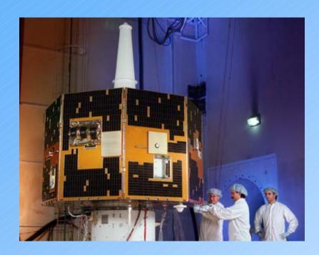
IMAGE designed as single string with only limited redundancy.
