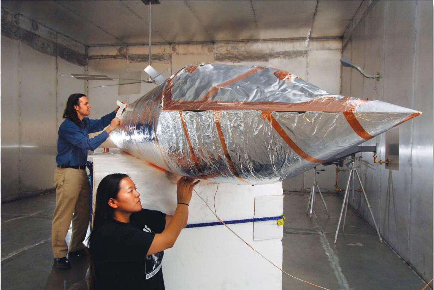
Staff prepare an Advanced Cruise Missile for testing in the large Mode-Stirred Chamber.
