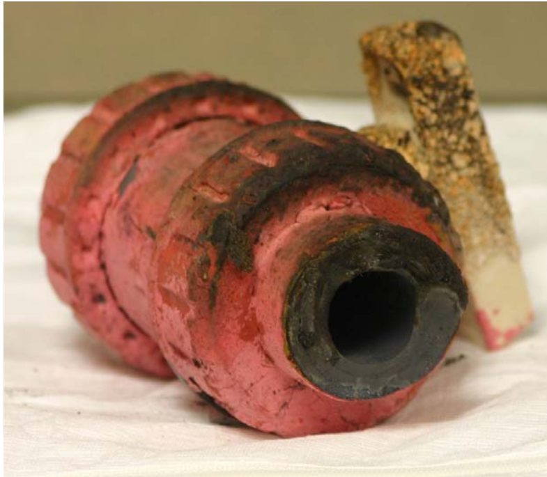
Figure 5. Failed 1-inch PVC pipe showing fracture surface
