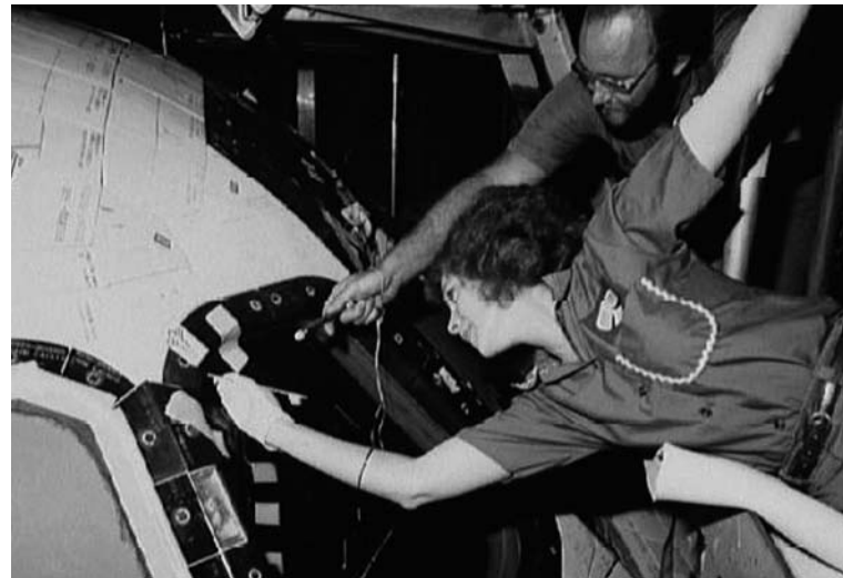
Technician Pat Klose leans over an edge in order to repair one of the protective thermal tiles on the Space Shuttle Columbia , prior to its fourth launch in 1982.
