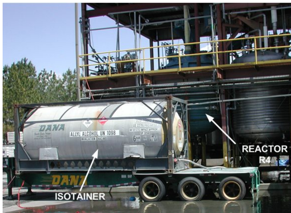
Figure 2. Isotainer (tanker) used to ship 35,000 lbs of allyl alcohol (looking east).
