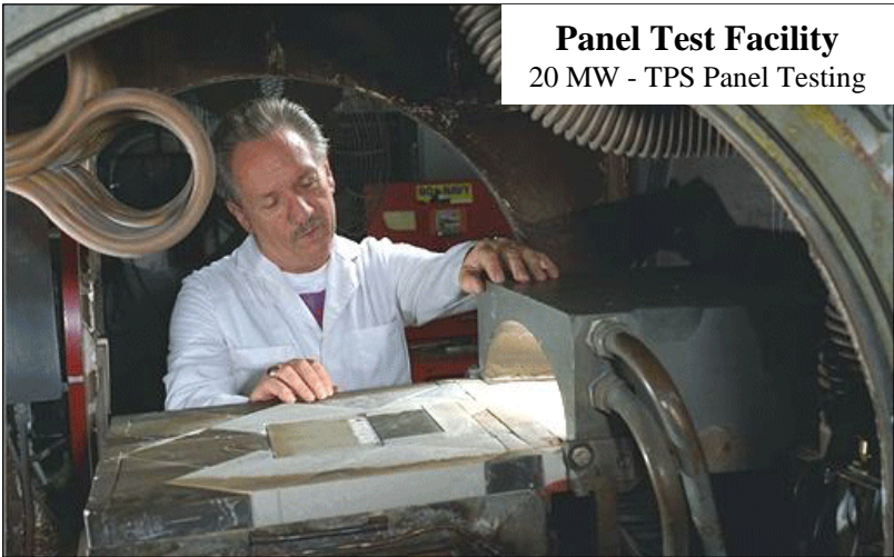
2"x9" Turbulent Flow Duct 20 MW - TPS Panel Testing
