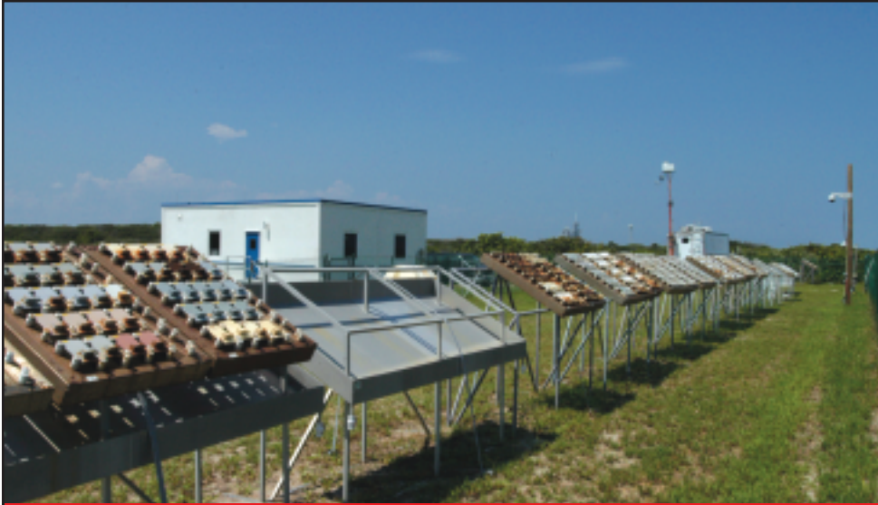
COATED PANELS UNDERGO RIGOROUS TESTING AT THE KSC ATMOSPHERIC CORROSION TEST SITE. THE FACILITIES AT THE CORROSION TECHNOLOGY LABORATORY ARE AVAILABLE TO COMPANIES AND INDIVIDUALS OUTSIDE OF NASA. THEY CAN PROVIDE A WAY FOR THE FINISHING INDUSTRY TO ADVANCE CORROSION-RESISTANT TECHNOLOGIES.
