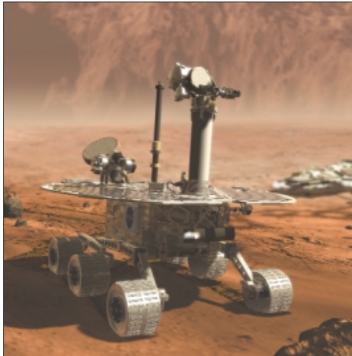
The two Mars 2003 rovers will extend the surface exploration begun by Viking and Pathfinder. These new rovers will be able to travel 100 meters per day, and will carry scientific instruments to determine the geological context of rocks and soil and measure their chemical composition and fine scale structure—even scraping the surface off rocks to expose their unweathered interiors.
