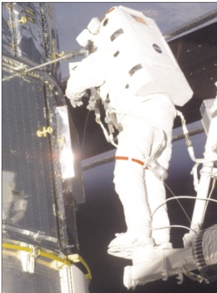
The Hubble Space Telescope (HST) was designed to be a serviceable spacecraft. An astronaut uses the Power Ratchet Tool on an HST bay door while replacing the observatory's flight computer.
