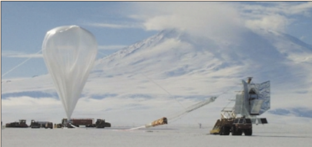
The BOOMERANG Telescope being readied for launch near Mt. Erebus in Antarctica. The 28 million cubic foot balloon carried the BOOMERANG telescope to an altitude of 120,000 feet, above 99 percent of the atmosphere.
