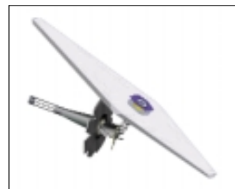
One possible concept for an NGST design, showing the telescope beneath a large Sun shade.
