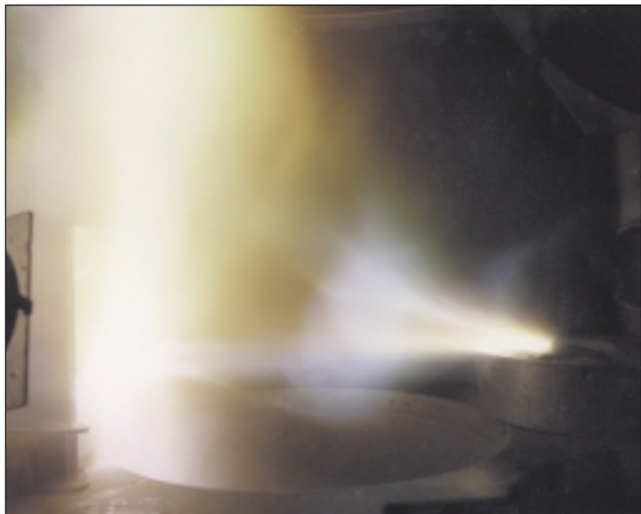
Time exposure of a hypervelocity oblique impact, from the right of the frame. Low-angle impacts cause the projectile to fragment, and significant pieces survive to disperse downrange without much change in velocity. (NASA Ames Vertical Gun Range)
