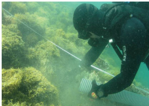
A Super Sucker device is used to vacuum alien invasive algae off coral reefs in Hawaii. source: Hawaii DAR
