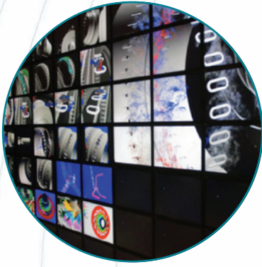
The 128-screen hyperwall-2 system is used to view, analyze, and communicate results from NASA's high-fidelity modeling and simulation projects, leading to new discoveries
