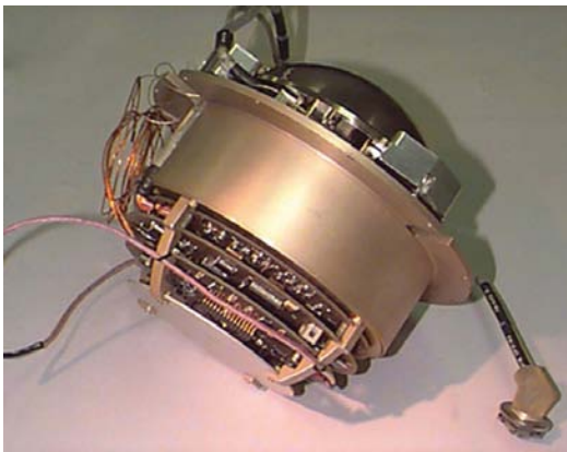
Main electronic subassembly of the new W76 Telemetry System.
