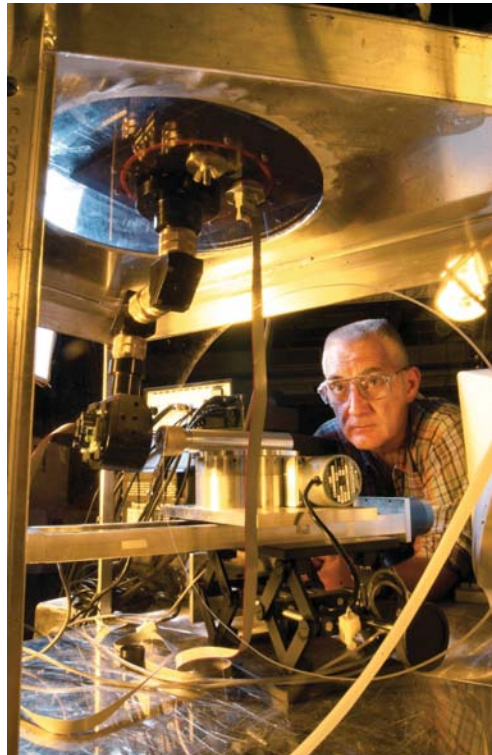
Scientist performs surface inspection using Diffuse Reflectance Infrared Fourier Transform (DRIFT) spectroscopy.
