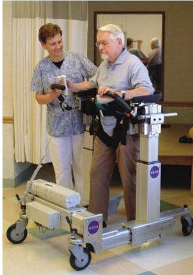
SAM (pictured) helps patients with a variety of injuries and diseases relearn to walk and perform physical therapy exercises.
