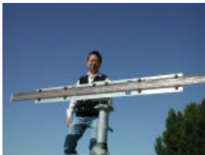
PR-2: Ku-band antenna feed array
