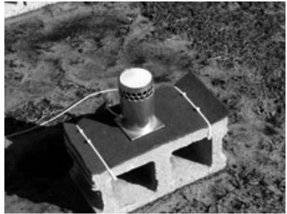
Disdrometers like this one measure rainfall rates and size distribution. Credit: NASA.
