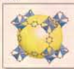
"Isoreticular" IRMOF-1: tunable pore size and pore chemistry (Yaghi et al., Science 1999)
