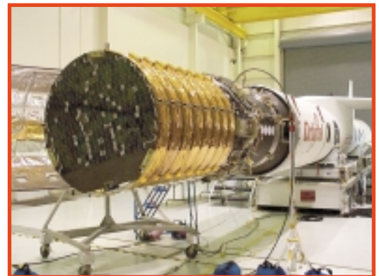
Eight ORBCOMM satellites mounted to Pegasus
