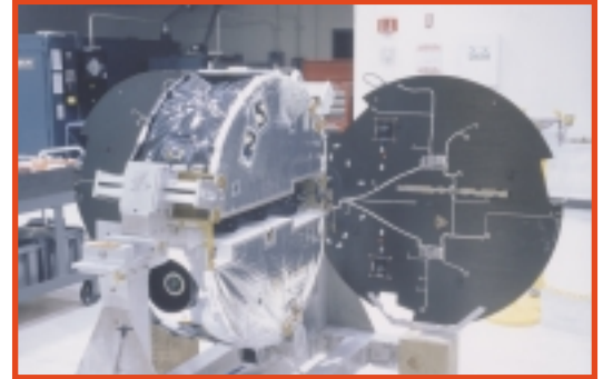
OrbView-1 (MicroLab) during integration and test
