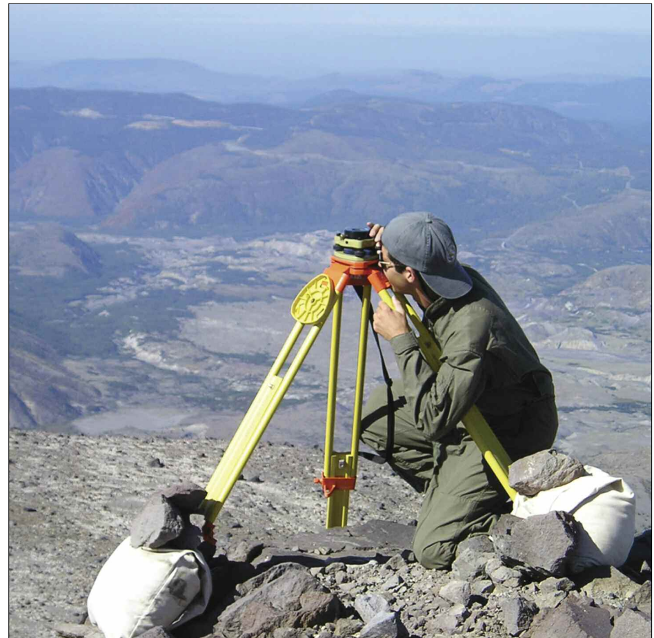
Global Positioning System (GPS) stations like the one above receive satellite signals to precisely capture movements in the Earth's crust. See the related story, "Earth's crust in action," on page 10. (Courtesy M. Lisowski)
