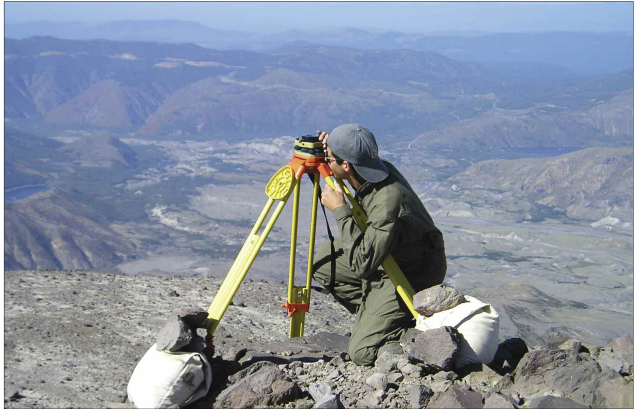
A researcher checks the calibration of a ground-mounted Global Positioning System (GPS) station on Mount St. Helens. GPS receivers and satellites can precisely capture movements in the Earth's crust, giving scientists a picture of processes concealed deep in the ground during earthquakes and volcanic eruptions. (Courtesy M. Lisowski)
