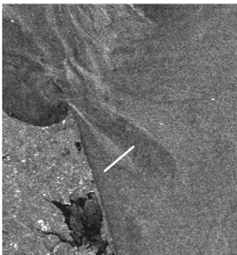
Figure 9. A RADARSAT-1 SWB image covering the Delaware Bay mouth region taken on 7 February 1997, 1115 UTC. The white line represents the transect along which gray level values are taken for comparison to the theoretical model.
