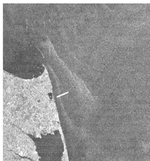
Figure 5. A RADARSAT-1 SWB image covering the Delaware Bay mouth region taken on 13 August 1996, 1107 UTC. The white line represents the transect along which gray level values are taken for comparison to the theoretical model.
