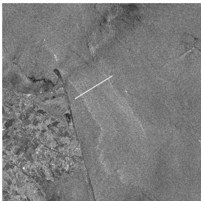
Figure 13. An ERS-2 standard image covering the Delaware Bay mouth region taken on 14 May 1997, 1543 UTC. The white line represents the transect along which gray level values are taken.
