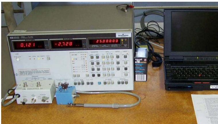
Figure 9 – Setup of the Virginia Tech SHM instrumentaton.
