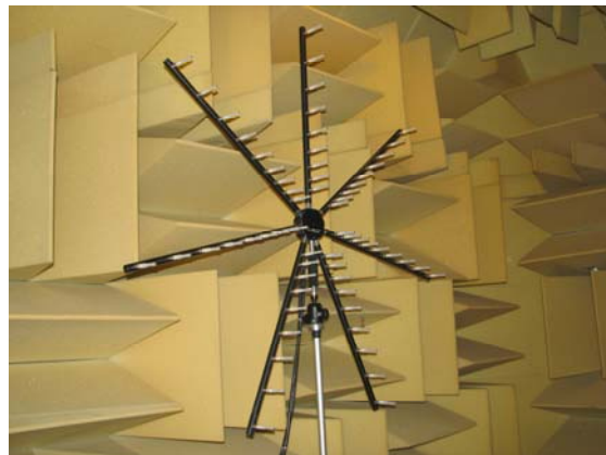
Figure 6: Microphone phased array.
