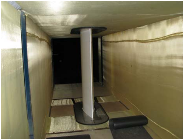
Figure 5: DU97-W-300 model in wind tunnel test section. View is upstream.
