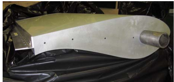
Figure 4: Flatback wind tunnel model with splitter plate attached.
