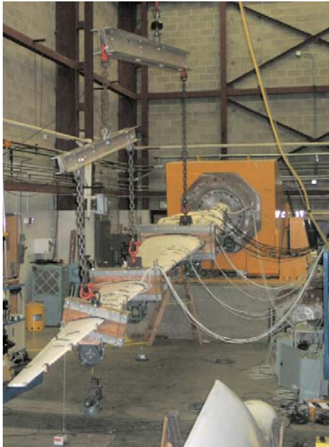
Figure 7. CX-100 blade in test fixture.
