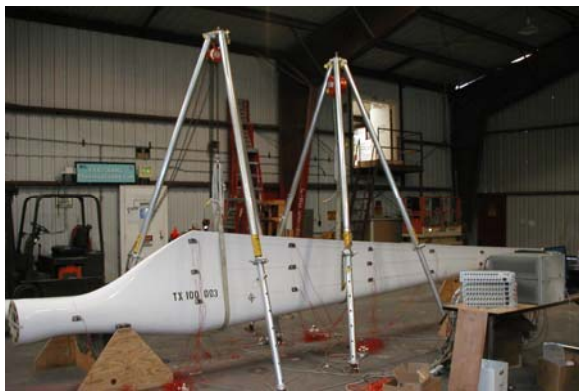
Figure 4. Double strap suspension configuration.
