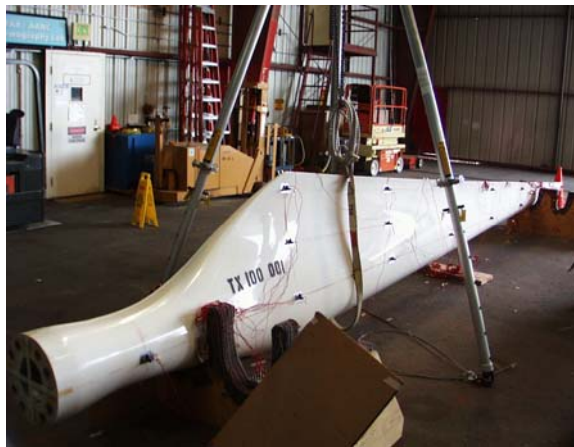
Figure 5. Single strap suspension configuration.
