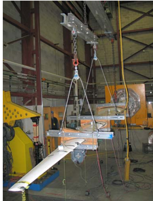
Figure 8. TX-100 blade in test fixture.
