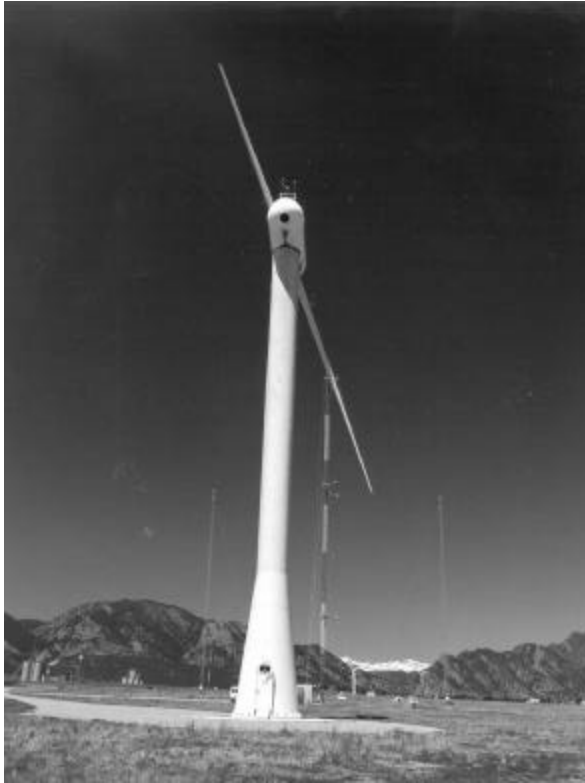
Fig. 1. NWTC LIST 42-m Inflow Measurement Array Upwind of ART Turbine and Looking Towards Prevailing Wind Direction.
