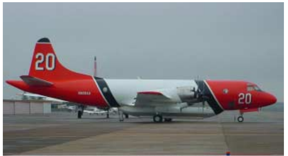
THIS P-3 ORION, a former Navy patrol plane modified to carry retardant, is part of the US Forest Service fleet of large air tankers for firefighting.
