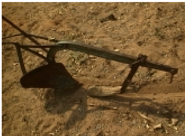
Traditional mouldboard plough which is the most common animal drawn implement but not necessarily good for soil and water conservation. Here it is shown with the furrow wheel replaced with a wooden sledge.
