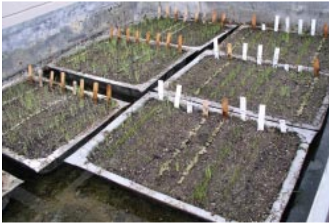
Figure 4. Artificial wetland tank with greenhouse flats.
