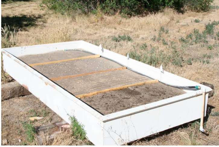
Wetland tank divided into 2X4' plots for treatments.
