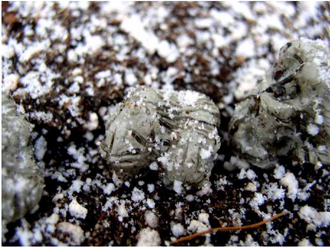
Figure 4. SS particle exhibiting ice fractures.
