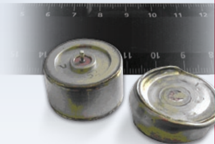
Heated to 250 degrees C and crushed under 60 tons of pressure, the battery at the right continued to function as expected.
