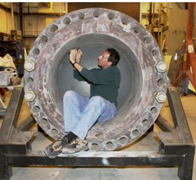
Richard Simpson, of Sandia's Applied Nuclear Technologies department, measures a weld in a 1/5 scale model pressure vessel lower head assembly.
