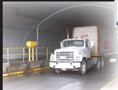
Above: VPED stand-alone user interface. Left: Radiation detectors interrogate passing vehicles
