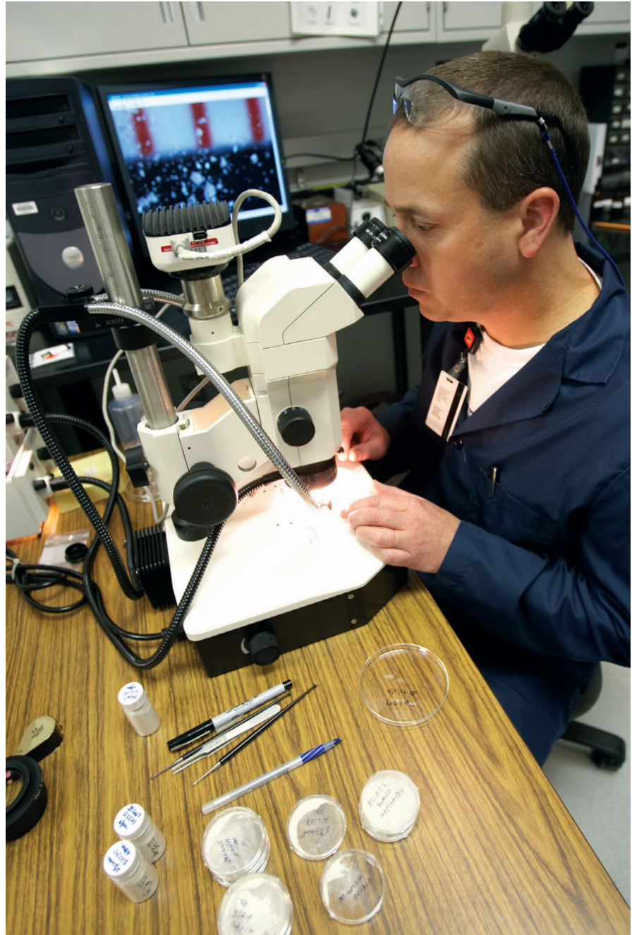
A scientist in FDA's Forensic Chemistry Center isolates foreign particles from contaminated wheat gluten using a stereoscopic light microscope. These particles will be analyzed using advanced analytical chemistry techniques.
