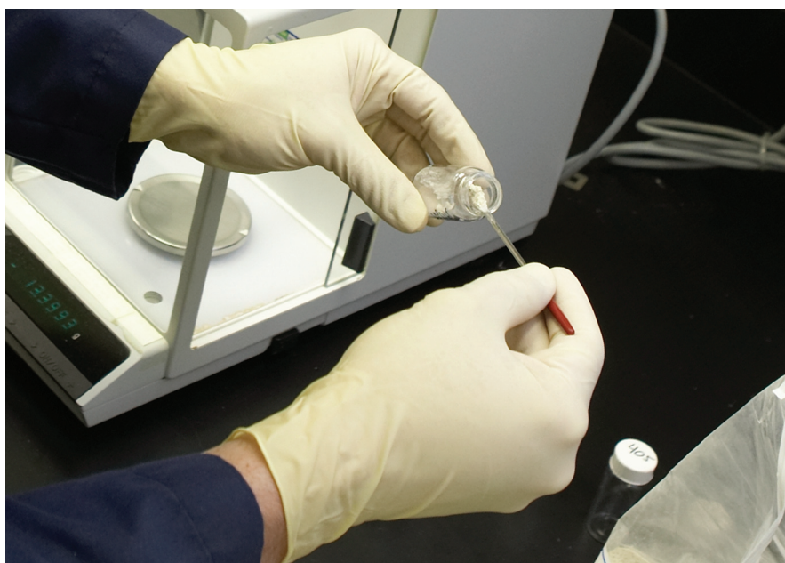
A scientist in FDA's Forensic Chemistry Center weighs out a sample of wheat gluten to be tested for melamine. Once the samples are prepared, state-of-the-art instrumentation is used to check for the presence of melamine contamination and to determine the amount present.
