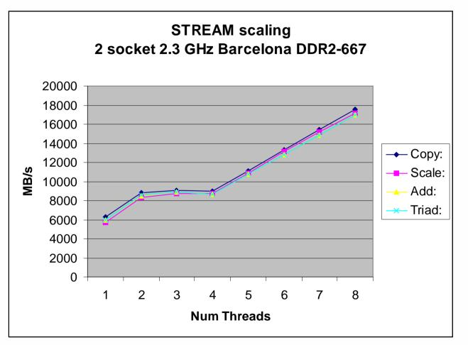
Supermicro H8DMU serverboard, Two 2.3GHz Barcelona cpus, 8 x 2GB DDR2-667 CL5 memory SLES10 SP1, Pathscale 3.1 C compiler
