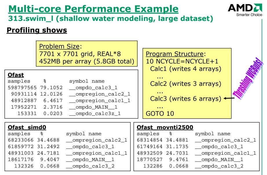
Oprofile: Counted CPU\_CLK\_UNHALTED events (Cycles outside of halt state)
