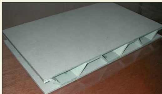
Engineered structural panels can be made by using simple uniaxial core structures to provide efficient structural panels. The panel shown is approximately 1-1/2 inches thick.
