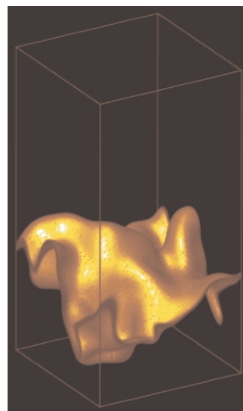
Figure 26. Combustion simulation of turbulent flame, showing surface of maximum heat release.
