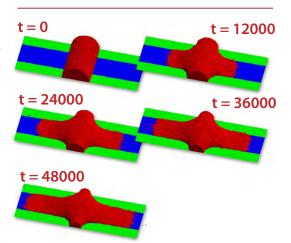
Snapshots from simulations of a polymer nano-droplet (red) spreading on a chemically patterned surface. The pattern consists of parallel strips of alternating wetting (blue) and non-wetting (green) regions. The droplet spreads on the wetting strip by removing material from on top of the non-wetting region. Understanding wetting on complex patterns will guide the way to engineering material delivery to specified device areas.
