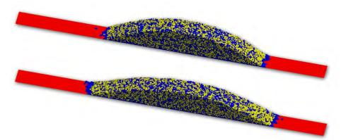
Snapshots at two different times from simulations of binary component polymer nano-droplets. The wetting constituent (blue) forms a monolayer on the surface (red) and spreads outward. Subsequently, the non-wetting constituent (yellow) spreads on top of the wetting monolayer.
