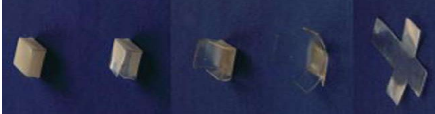
Figure 1. Photo sequence demonstrating the thermally induced shape memory effect for a poly (ε-caprolactone dimethacrylate) polymer. Starting from room temperature, the polymer, in its temporary shape (cube, left) is heated up to 70 °C, which is above its glass-transition temperature. Within 60 seconds, the sample recovers its permanent shape, which is a nearly planar film (right). Reproduced from Lendlein, A. et al. Encyclopedia of Materials Sci. and Tech. , 1-9.
