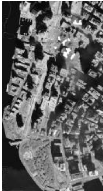
NASA's September 16 AVIRIS flight over Ground Zero (upper right) at mid-day revealed dozens of thermal "hot spots" with temperatures as high as 1,300 degrees F. In this image, areas with the highest recorded temperatures are shown as white patches. Analyses of AVIRIS data also showed composition of airborne particulates.
