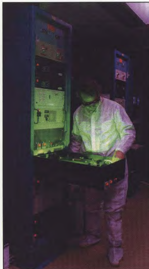
A technician works with the diode-pumped solid-state green laser developed for U-AVLIS. The technology is being used for precision machining and many other applications, such as pumping ultrashort-pulse lasers, creating laser displays, and treating disfiguring skin conditions.
