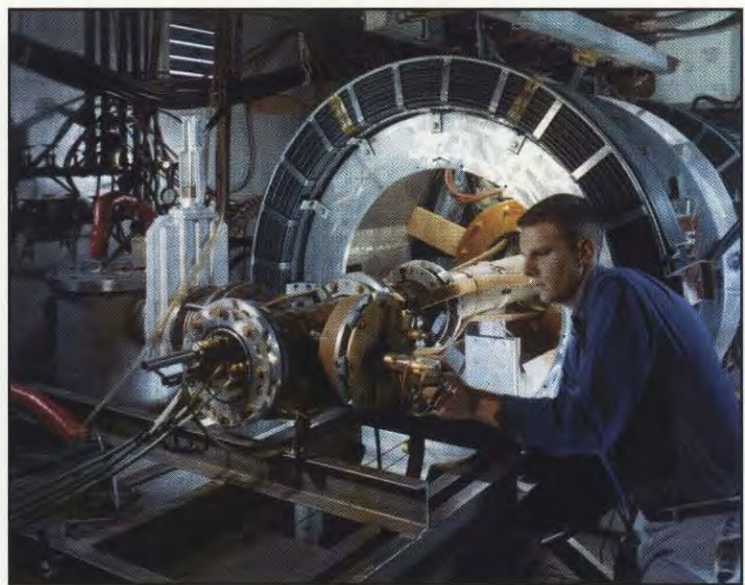
An early fusion research device called Toy Top was used to create a hot, mirror-confined plasma by plasma injection and magnetic compression. Toy Top experiments succeeded in producing fusion neutrons, a significant early achievement in the controlled fusion program.
