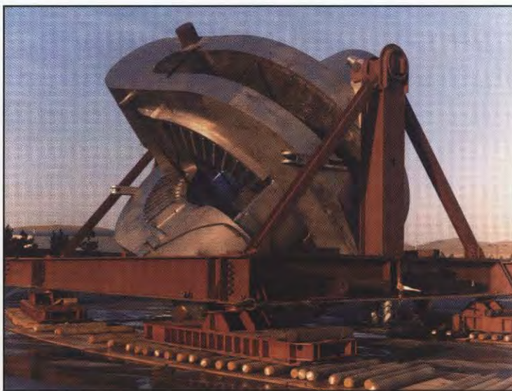
One of the yin-yang magnets for MFTF-B being moved into Building 431. The magnet system for MFTF-B was the largest superconducting system ever built.
