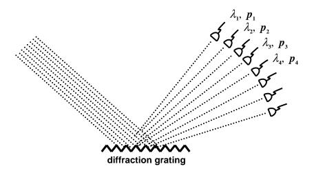
A diffraction grating disperses waves of different wavelengths, and therefore different momenta. Detectors arranged as shown will produce a histogram of clicks for different momentum components present in the incoming stuff.
