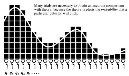
Each square corresponds to a single click in the detector below it. Schrödinger's wave amplitude (squared) predicts the curve through the tops of the columns of squares.
