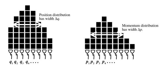
Schrödinger waves can appear in "position space," or "momentum space," or whatever quantity the detector array is set to measure. The two sets of detector clicks shown have characteristic spreads conventionally denoted  $\Delta q$  and  $\Delta p$ .
