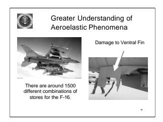
To underscore the importance of modeling very complex flow fields. This F-16, with its large complement of stores behaves very differently than the idealized configuration that can be analyzed with today's techniques and computing capability.
