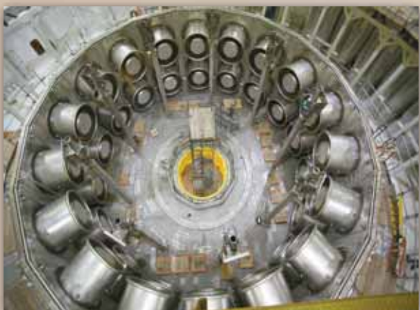
Z machine's center during the renovation process, its huge conduits being readied to focus an even more massive electrical current on a target
