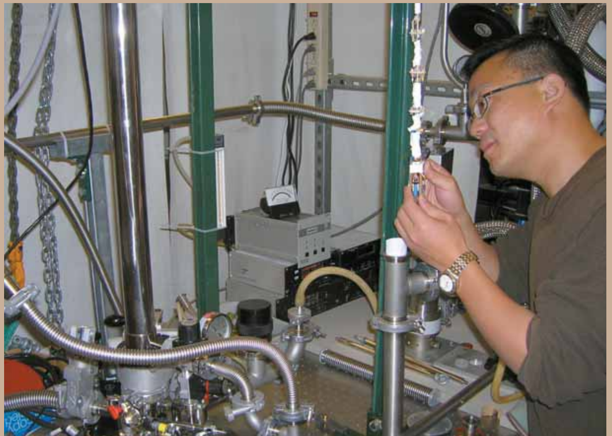
Sandia physicist Wei Pan prepares a sample for cooling to millikelvin temperatures in a magnetic field of 140,000 Gauss, where non-Abelian properties of novel electron-based particles can be observed.
