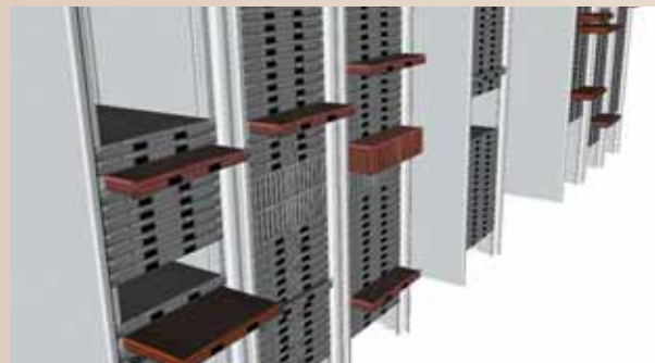
Portion of the OVIS-2 three-dimensional interface. Components with outlier behavior are indicated by color and distance projected out from the racks.
