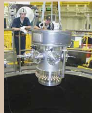
A successfully contained hazardous material experiment being removed from the Z machine's center section
