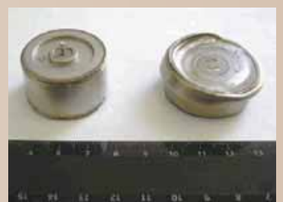
Prototype batteries. One was heated to 250°C and then crushed to demonstrate the battery's safety.
