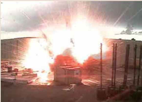
The expanding fireball from a Sept. 6, 2006, Reliable Replacement Warhead hydrotest at Los Alamos National Laboratory's Dual Axis Radiographic Hydrotest (DARHT) facility is shown a fraction of a second after detonation. Center 2400 personnel built critical components used in the test.
