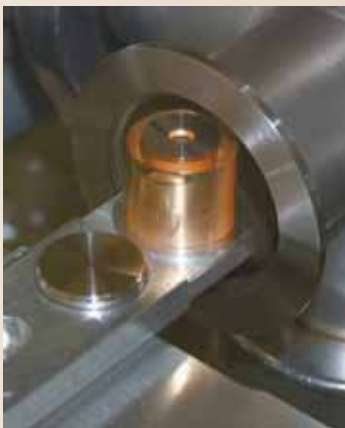
Assembled micropower source ready for testing at Oak Ridge National Laboratory
