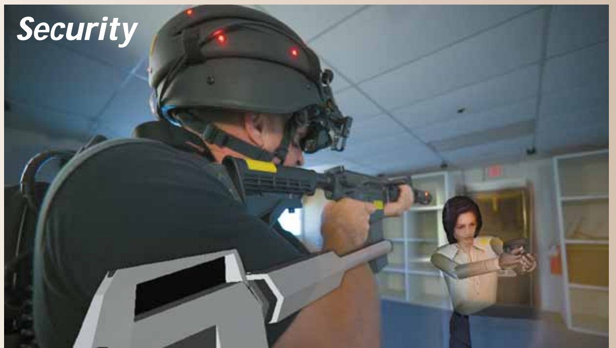
Trainee using the Augmented Reality Training System (ARTS), an immersive virtual training system where multiple ProForce officers can exercise their tactics against virtual bad guys who emerge from real corners and fire back at them
