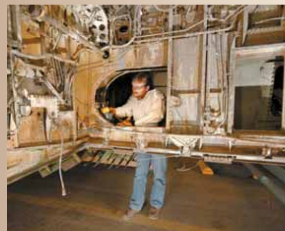
KEVIN HOWARD inspects the wiring in an aircraft landing gear bay. (Photo by Randy Montoya)
