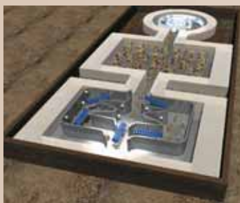
Artist's conception of an integrated sensor device. In the foreground is the analyte capture section; in the center section the analyte is tagged with quantum dots; in back they are collected for detection.
