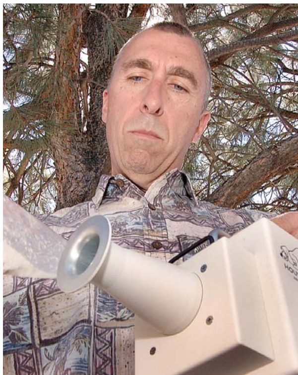
DAVE HANNUM demonstrates the drug-sniffing capabilities of the Hound handheld sniffing device. (Photo by Randy Montoya)
