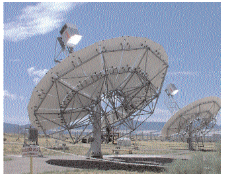
SOLAR THERMAL systems are becoming a viable power source in remote areas for water-pumping and village electrification.
